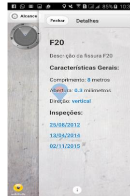
Figure 5: Screen showing crack details.
